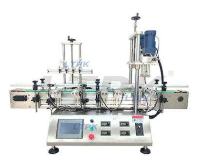
This machine adopt stainless steel magnetic pump, corrosion resistance, the machine combines the filling station and the capping station together to realize inline filling and capping work, compact machine body saves working space. It can work with tabletop labeling machine to realize automated packaging work.
