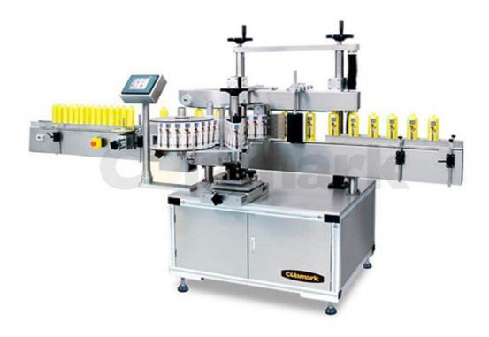
A910 is an ideal choice for the cosmetic, food and beverages, pharmaceutical and other light industries automatic side labeling on oval shaped or rectangular shaped containers. Wrap-around belt, pneumatic wrap-around station and turn-table wrap-around station is optional for wrap-around labeling on the round bottle.
