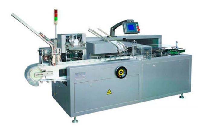
This machine is suitable for cardboard case packaging of blister package for blister package and similar package. It consists of direction folding (1-4 folds) and feeding equipment, cardboard case forming and feeding, batch number printing, sealing of case tongues at both ends etc. The whole encasing process is finished automatically. It can be added hot-glue machine.
