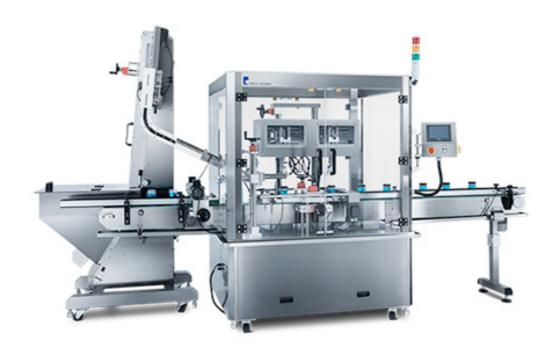
The Pack Leader CCP-132 is an innovative, fully automatic capper which benefits a wide variety of companies requiring capping capabilities. The machine's triple servo driven system controls the capping function to ensure that the caps are the proper tightness so the product meets perfection when it is presented to the market.
