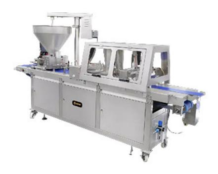
ANKO's elaborate burrito machine is recommended for automating the burrito wrapping process. Simply by putting a tortilla in position, as it's detected by sensor, the burrito machine automatically deposits quantitative filling on it. Up to 1,000 appetizing burritos are able to be formed in an hour. The productive machine not only saves labor costs, but also enhances quality and capacity.
