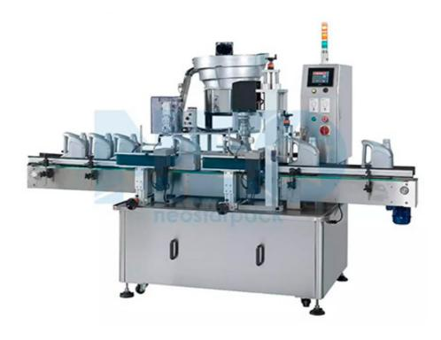
Automatic Capper CC4170 can be easily adjusted with the capping head to meet different capping requirements. With dual clipping conveyor, all kinds of bottles can meet precise position while caps feeding and capping.
