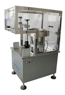
In the automatic bottle feeding process, the cap manager cap system is continuously transported to the position of the cap, and accurately set on the mouth of the bottle, the cap device will press the cap in the mouth of the bottle, complete the process of pressure inside the cap.
