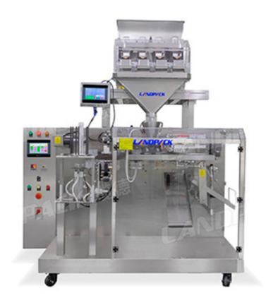
Automatic granules horizontal premade pouch packing machine, it is suitable for the measurement and packaging of various fine particle products, such as sugar, salt, chicken essence, monosodium glutamate, buckwheat, snacks, etc. After replacing the metering device, it is suitable for packaging liquid and powder products.
