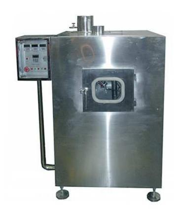
The machine is used to carry out sugar coating and so on to the core of Chinese traditional medicine and western medicine tablets, it integrates strong power, weak power and hydraulic pressure with pneumatic operation, it is new type equipment improved on the basis of original common type sugar coating machine.
