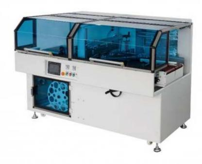
Shrink wrap machines apply heat to shrink a plastic film around a product. This process is often done by automated equipment, but manual and semi-automatic shrink wrap machines are also available. Shrink wrap machines cover the item, and then sent it through a heat tunnel or oven for shrinking.
