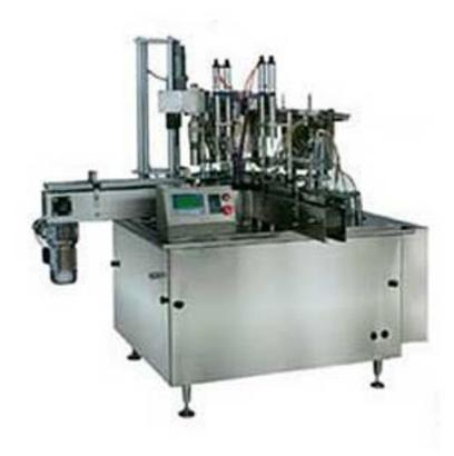
The SD-YYS-170 filling sealing machine (filler sealer) is suitable for the high output production of eye drop. It can work with high speed but also stably and is of high eligibility rate. This equipment can be also used to produce iodine, 3essential balm and tincture.
