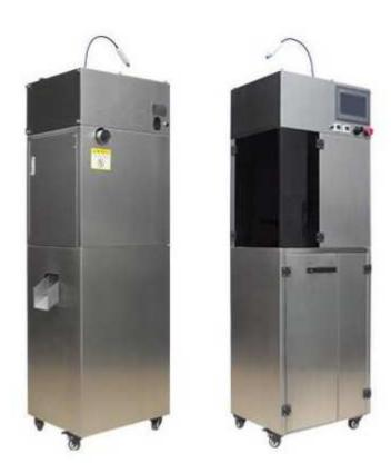
In the relatively airtight environment-working cabin, use high and low pressures to alternate changes rapidly "pressure shear" causing pulsed drawing force to the capsule. Under the continuous function of the pulsed drawing force, the capsule is gradually drawn and separated.
