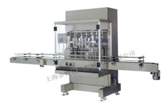
The BGF series weight/injection filler is a high-tech product designed and developed by our company. It mat suit for different viscosity of water agent, semi-fluid and paste, it is widely used in the product filling of foodstuff, cosmetics, medicine, grease, daily chemical industry, detergent, pesticide and chemical industry. Using the straight filling way, may be used in the different vessels, needn't add any parts.
