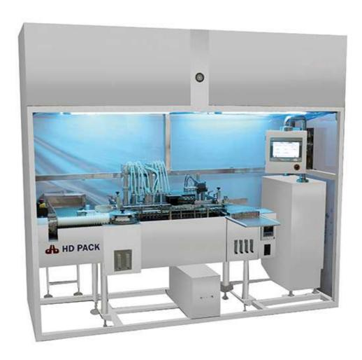
This machine is constituted of multi-stations step by step conveying system and balcony type structure. It can carry out the procedures such as ampoules conveying, front gas charging, filling, rear gas charging, preheating and welding. The machine has been designed, following the strict criteria typically needed in aseptic environment such as minimized diameter, the geometry facilitating the unidirectional airflow, high ergonomic level and compact design.
