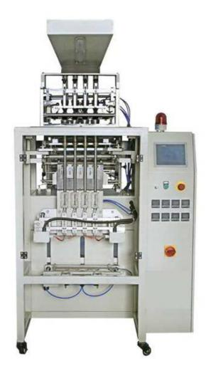
This machine can be made special for the customer requirement from 2-8lines.the bag length can be set discretionary inside the standard range without change any device.
