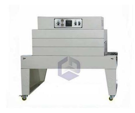
BS-A450 thermal shrink packaging machine is suitable for shrink films such as POV, PVC, PP, POF, etc. There are shrinking tubes on the top, bottom and sides of the shrinking room. The temperature of the shrink room and the speed of the conveyer are adjustable. And the size of the machine can be customized.
