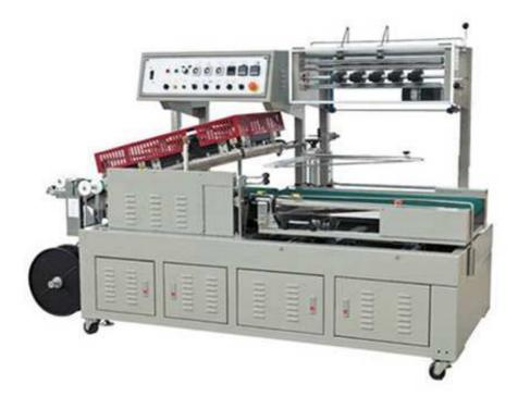
Traditional Middle speed L bar sealer has no reciprocating sealing function, so the sealing line is not strong enough and has the holes or welding seams after shrinking. The new model of TY-703-150H-ST is designed to avoid these problems.
