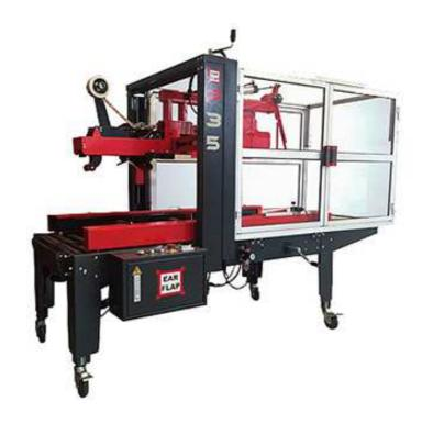
The P35 Carton Sealer is a single format carton taping machine that is capable of taping cartons up to 480mm in width and 480mm in height and 700mm length. It can tape both the top and bottom of a carton and has some manual adjustment. It has an option for a hot melt sealing system. The P35 Carton Sealer is designed and manufactured by respected Spanish company Ear-Flap and is available exclusively in Australia from Australia Engineering.
