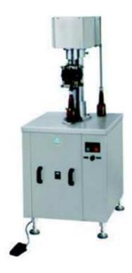
Semi Automatic Capping Machine is precision built on sturdy welded steel frame completely enclose in stainless steel sheet and doors are provided to facilitate the servicing of machine. Machine is motorized incorporating rotating threading & sealing rollers, for threading & sealing of ROPP cap.
