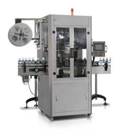
All-cover type stainless steel host machine: the whole machine is waterproof as well as rustproof. Adjustable cutter head: unique cyclotron cut-off, double sided cutting edge with a long service life. Single positioning centre guide pillar: more stable for label delivery.
