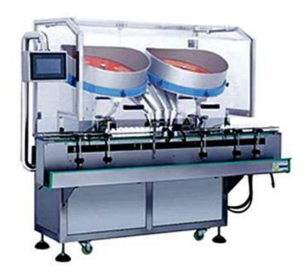
Double-head counting machine is suitable for pharmaceutical, food, and chemical industries. It automatically fills bottles with pills or tablets, then counts and covers the bottle. It can be connected with next process. Being beautifully designed and easily regulated. It is an ideal choice for packing for packing and counting equipment.
