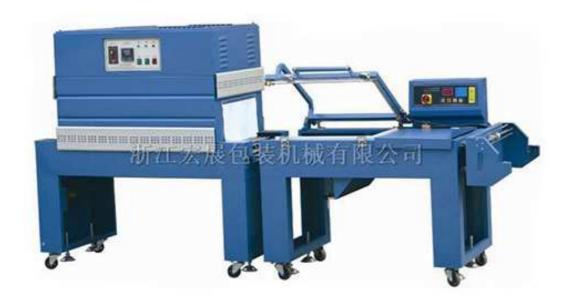
Shrinking machine with L-BAR realer is suitable for electrical, hardware, software, food, printing products, medications, floor boards, ceramics etc. Suitable for PVC, POF, PP film's using.
