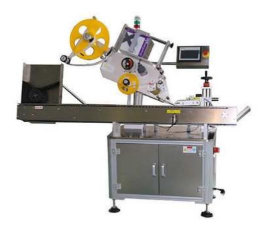
Applicable for round objects with smaller diameter which cannot stand when labeling, such as ampoule, vials, blood collection tube, pen, sausage and so on. (P.S. our labeling machine can be designed according to your needs)
