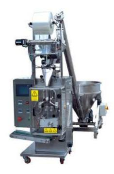
This machine can be used to pack all kinds of free-flowing powder materials such as flour, coffee powder, starch, soymilk powder, bone-strong powder and nutritious food stuff in powder form etc.
