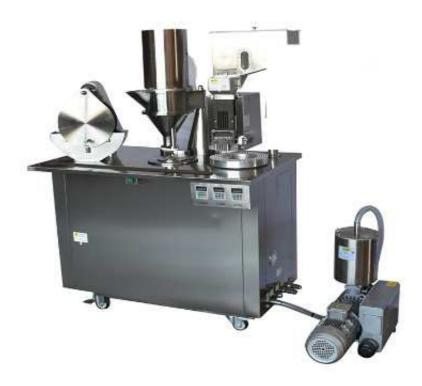
Packry's Semi-auto Capsule Filling Machine (CGN208-D) is widely used by small and medium pharmaceutical companies, such as hospitals and small laboratories. The machine adapts programmable control system, colorful touch screen, automatic capsule counting. The machine is automated by the section including capsule positioning, separating, filling, locking.
