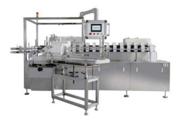
This machine is suitable for cardboard case packaging of tube toothpaste, foods, sachets, ointment, and soft package (packed condoms). It consists of direction folding (1-4 folds) and feeding equipment, cardboard case forming and feeding, batch number printing, sealing of case tongues at both ends etc. The whole encasing process is finished automatically. It can be added hot-glue machine. It is favored by domestic and foreign companies.
