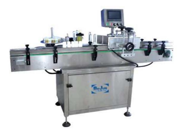
The machine suits for label of the cylindrical vessel, can once only complete label-sticking and packing up. It uses photoelectric detecting and synchronous tracing, ensuring synchronism of label-conveying speed and bottle-roaring, making label's sticking and pressing level.
