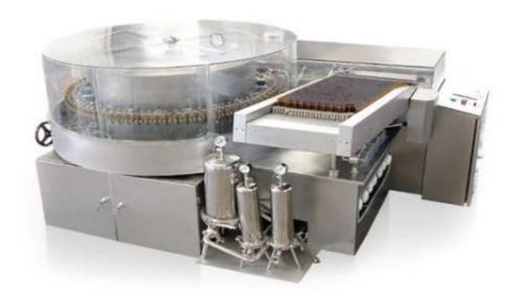
This machine is used for washing bottle and container in pharmaceutical, chemical and food industry and can complete the following procedures: conveying bottle automatically, ultrasonic washing, flushing with air, water alternatively, outfeeding bottle automatically.
