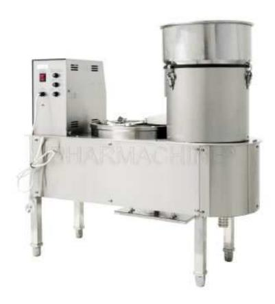
This machine has been designed and developed to count & fill different shapes or size of products accurately like soft gel capsules, hard capsules, tablets, sugar coating, and film coating tablets, pills, herb medicine or similar products into containers or vials.
