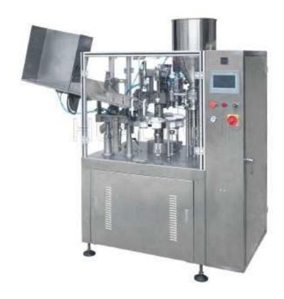
This machine adopts PLC controller and color touch screen are applied and made it possible for programmable control of the machine. It can perform the filling for ointment, cream jellies or viscosity material, tail folding, batch number embossing (include manufacture date) automatically.
