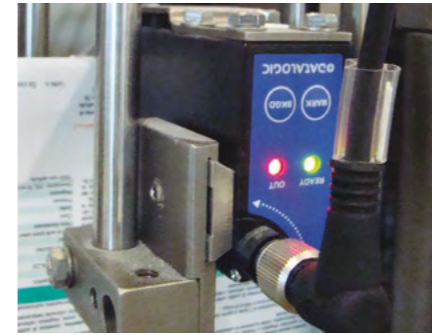
Adjustable photocell to read the eye-mark in any position.
