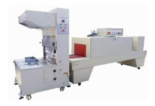
Semi automatic sleeve shrink wrapping machine can be used for bundle shrink wrapping. It's wildly used for beverage, can, bottle, cartons and more.
