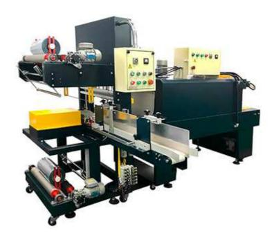
Sleeve-type Sealer with Tray Model, SSA1400 & SSA-1600 has PLC control system can detect film running and alarm of trouble to indicate problem helping technician fix machine easy.
