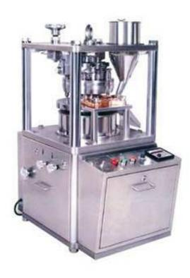
Lab Tablet Press Machine is used for production of simple and precise tablets from powder in Pharmaceutical and relevant Industries for research & development.
