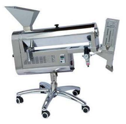
NFJ-150 Capsule Polisher is a kind of capsule polisher with function of sorter as well. It plays the function of polishing capsule. It can also automatically reject low weight capsule, loose piece and fragments of capsules. It is suitable for all sizes of capsules without the need to change parts.
