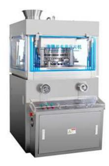
ZP25 effervescent rotary tablet press machine is a latest rotary tablet press developed by our company, used to press granular raw materials into tablets. It is the only professional effervescent tablet press in china. It is mainly used for tablet production of effervescent tablets, aromatic tablets, washing blocks and other tablets with difficult mold release.
