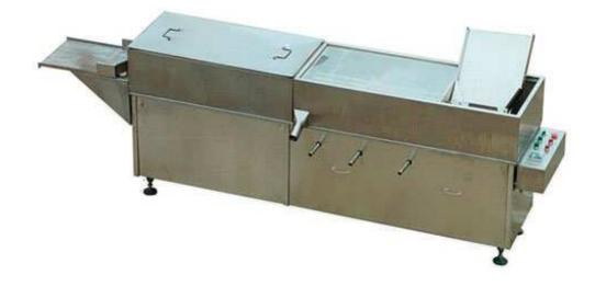
This linear cleaning dryer is mainly used to wash and dry oral liquid bottles without needs to be sterilized, and bottles treated by this dryer can be filled directly.
