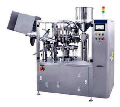
This ointment tube filling and sealing machine is widely used for different hoses (various plastic pipes with different diameters of  $\Phi$ 16- $\Phi$ 35, aluminum-plastic composite pipes), as well as filling materials with viscosity and characteristics (from water to high viscosity paste). Installation, fully meets the requirements of different levels of GMP production environment.
