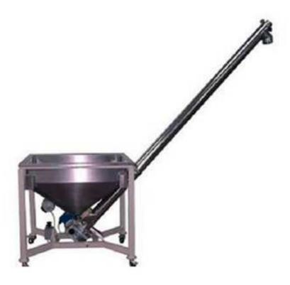
The product is mainly used as a granular powder feeding, suitable for food, chemical industry, building materials, plastics and packaging industry has a certain height requirements of the feeding device.
