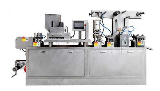
Blister Packing Machine DPP-140 is specially designed for hospital dosage room, laboratory institute, health care product, middle-small pharmacy factory, and featured by compact machine body, easy operation, multi-function, stroke adjustable, long durability etc. It is suitable for the Alu-PVC package of medicine, food, electric parts etc. It has aided forming Pre-cutting Inspection and rejecting control systems, with print mark registration Automatic feeder.
