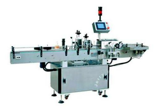
JTB-150A Automatic Stickers Labeling Machine is controlled by the PLC, HMI and servo drive labeling. The machine is easy to operate and has helping function and fault indication function. It is suitable for the self-adhesive labeling of round bottles.
