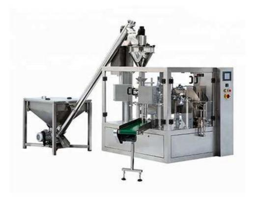
This set of equipment is mainly suitable for automatic packaging of prefabricated bag powder products, which consists of fully automatic rotary bag packaging machine, screw powder filling machine and screw hoist.
