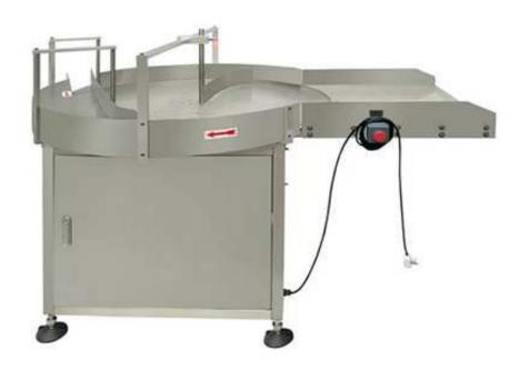
This machine is an auxiliary device in the production line. It is mainly used for storage, finishing and feeding of glass bottles to the production process.
