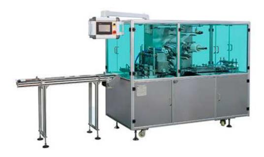
This type machine use BOPP or PVC transparent cellophane material to over wrap different size paper folding carton. Transparent cellophane stick with printed or laser tear tape make finished package easy open and has anti-fake function.
