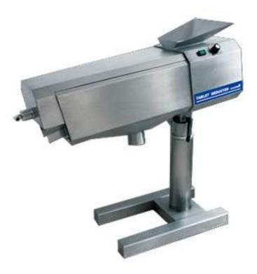
The high-speed tablet deduster model C&C200Badopts the principle of compressed air purging, centrifugal dedusting and roller deburring and vacuum extraction to clean the powder attaching on the surface of the tablet and burrs on edges so that the surface of tablet is clean and the edges are regular. It is a must have equipment in tablet production processes.
