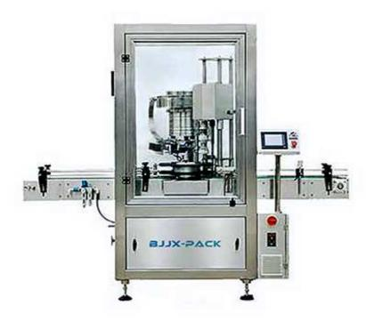
This machine adopts the design of vibrating cap sorter and fetching cap supplier. The capping head takes the cap and then capping which guarantee the qualification rate of capping. It can realize the capping of plastic caps, aluminum caps and press-in type caps in changing different capping device. It is easy to replace and operate. Capping for different containers can be replaced in a short period of time.
