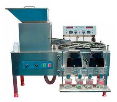
This is one kind of semi-automatic electric bottle counting and filling machine, it is desk type and easy to count and fill any shape of tablet or capsule into bottles. The most features is that no need to change any parts when you want to fill different shape tablets or capsules.
