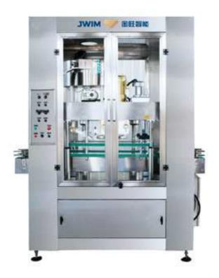
This automatic capping machine is used for closing screw caps, it is made up of 3 parts: cap feeding system, cap loading system, and cap closing system.
