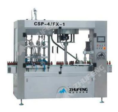
The product is a two-in-one machine which involve filling and capping two function. It suits for viscous material, simple structure, convenient operation, accurate metering and with high acceptance rate of lid-revolving.
