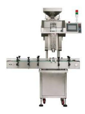
DI-200X Pre-cut Pouch & Canister Desiccant Inserter is new generation inserting system, which could put Pre-cut Pouch & small Canister or sieve drum into container. It is economical and easy to operate. The machine can automatically count pieces and insert it into the container accurately and speedy.
